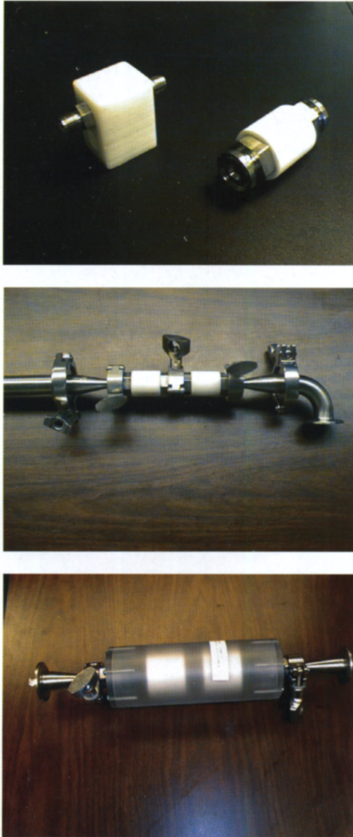
FIG. 6. Co-field flow PEF treatment chambers for benchtop and pilot plant-scale PEF system using stainless steel electrodes (top), a PEF treatment chamber for pilot plant-scale PEF system using stainless steel electrodes (middle), a PEF treatment chamber for pilot plant-scale PEF system using boron carbide electrodes (bottom). See Plate 1.
